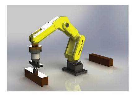
Motion studies are graphical simulations of motion for assembly models. They simulate and animate the motion you prescribe for a model. You can use SOLIDWORKS mates to restrict the motion of components in an assembly when you model motion.
